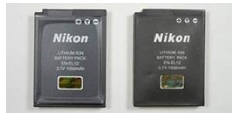
Comparison of authentic (left) and counterfeit (right) EN-EL12
